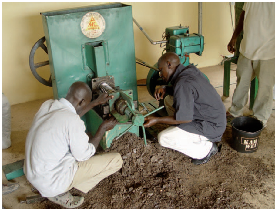
Workers in Garalo, Mali, press jatropha seeds that contain an oil that can be burned to produce electricity.
