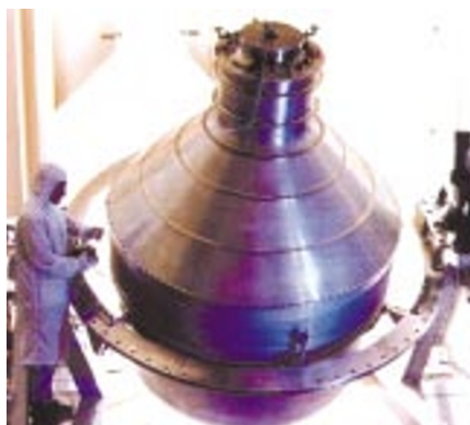
Getting warm: the dewar housing the gyroscopes may lose its cryogenic helium too quickly.
