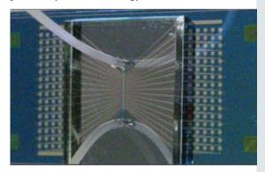
The device (pictured), developed by Aleksandr Noy at the University of California, Merced, and his colleagues, uses a carbon nanotube to bridge two metal electrodes. The nanotube is coated by a lipid bilayer. Embedded in that layer is the ATP-powered pump, which is widespread in cells and mediates the exchange of sodium and potassium ions across membranes. The central part of the carbon nanotube is exposed to an ATP solution.
