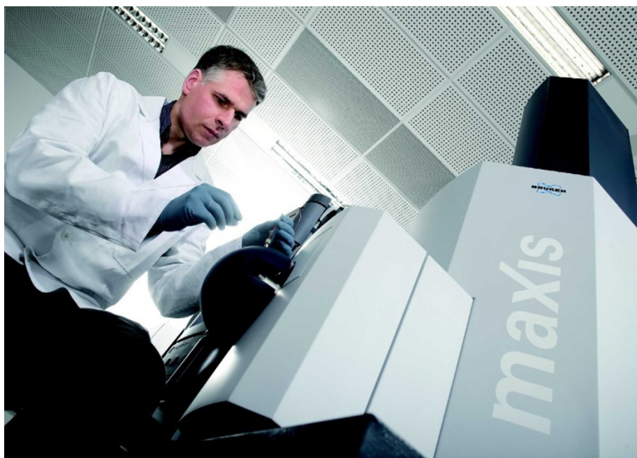
The maXis system from Bruker Daltonics can use both UPLC and CE separation approaches.
