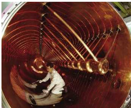
The GSI's UNILAC will serve as a pre-accelerator for a planned double-ring synchrotron.
