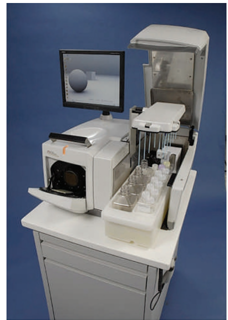
The Genome Sequencer FLX, developed jointly by 454 Life Sciences and Roche Applied Sciences, is based on 454 sequencing technology.
