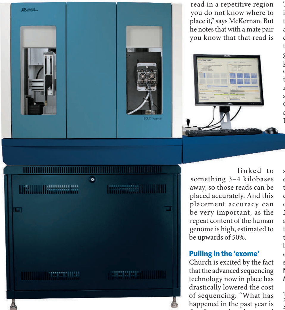
The next-generation SOLiD system from Applied Biosystems uses ligation-based sequencing methods.
