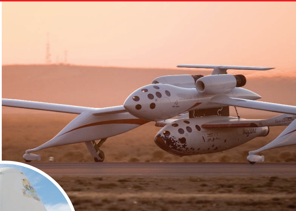
Different directions: unlike SpaceShipOne’s (above, with its carrier) horizontal positioning, New Shepard takes off and lands vertically.
