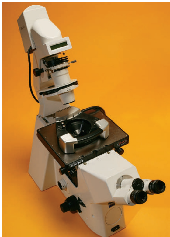
Two in one: the BioScope II combines atomic force microscopy with fluorescence microscopy.
