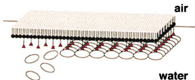
Figure 4 Two-dimensional protein crystallization on lipid layers. Schematic shows the binding of a protein of interest (oval objects) to the head groups (red triangles) of lipid molecules in a monolayer at the air–water interface. Rapid lateral diffusion of the lipids leads to protein crystallization
