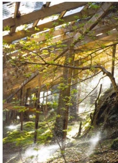
A plastic canopy protects trees in Gårdsjön, as part of an experiment to test the effects of nitrogen.
