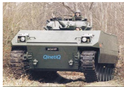
War machine: QinetiQ is known for its defence research, such as the design of this plastic tank.
