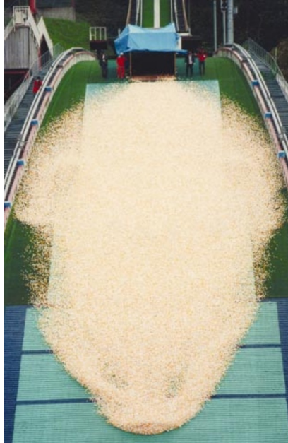
Rolling, rolling, rolling: thousands of ping-pong balls simulate an avalanche on a ski jump.
