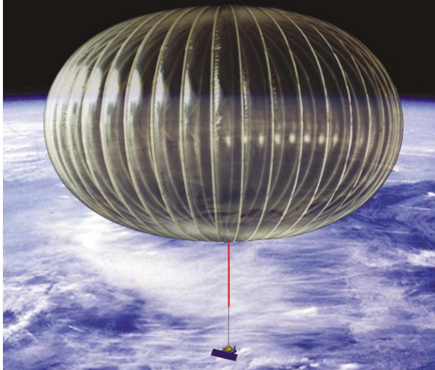
Smashing pumpkin: astronomers hope that this balloon design will be able to fly for about 100 days.
