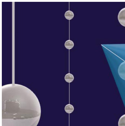
Simulation: strings of light-sensitive detectors in IceCube, one of two proposed neutrino projects.
