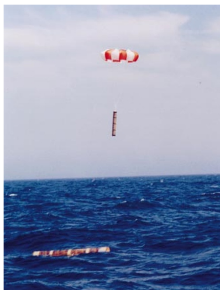
A drop in the ocean: water currents, temperature and salinity in remote areas are now being recorded by floats parachuted in for the job.
