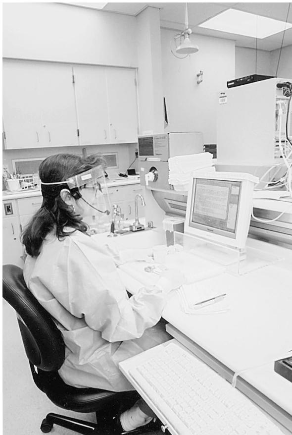
FIGURE 3. Pathologist assistant at voice recognition grossing station with space-saving arrangement as described in the text. The flat-panel monitor ( right ) also allows the monitor to be at eye level. The wireless headset microphone permits mobility without having to remove the headset. The receiver for the wireless microphone sits atop the PC unit ( upper right ).
