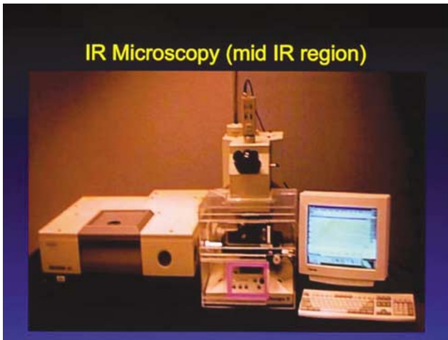
Figure 1 Mid-infrared spectroscopy system. For in vitro spectroscopic analysis, thick cryostat sections are placed in the spectroscopy specimen chamber (left). The territory of spectroscopic analysis is controlled robotically and matched to a hematoxylin- and eosin-stained frozen section placed on the microscope stage (middle). A computer station (right) completes the assembly.
