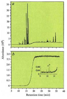
GC–MS chromatograms of samples of DDT milled with Mg: a, after 3 h milling; b, after 6.5 h milling. Cross, diphenylmethane; circle, diphenylethane. Measurements were carried out after extraction into n-pentane using a HP 5890 II GC–MSD 5790 instrument fitted with a DB-5 column of 30 m length, inside diameter 0.25 mm and film thickness 0.25  $\mu$ m. The carrier gas was helium at 70 kPa. The temperature programme was 40 °C for 2 min, then 15 °C per min to 310 °C and held for 20 min.
