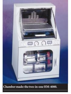
and all nucleic acid hybridizations. The lower chamber features temperature controls, variable rotation speed and multiple bottle size options, with rock-and-roll action available with an optional rocker plate. The upper chamber has a roller action to operate shaker tray or optional orbital tray.
