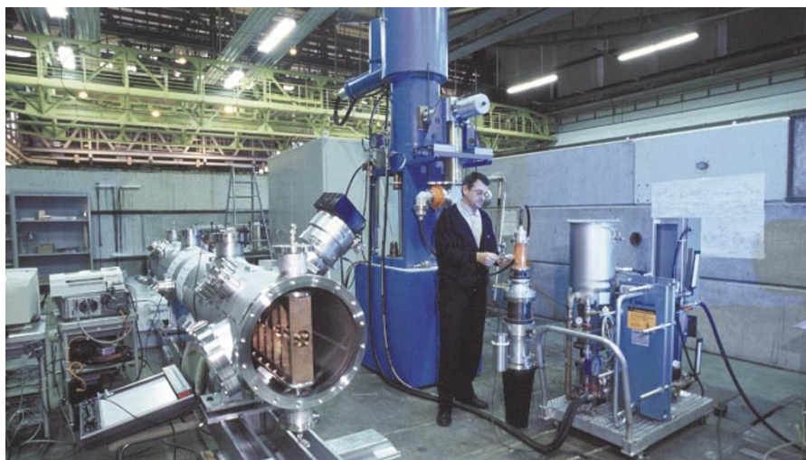
Braking system: the Japanese–European ASACUSA team will use this device to slow down antiprotons.
