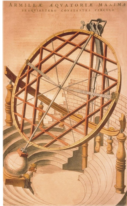
The 1585 equatorial armillary, the most versatile and impressive instrument on Hven.
