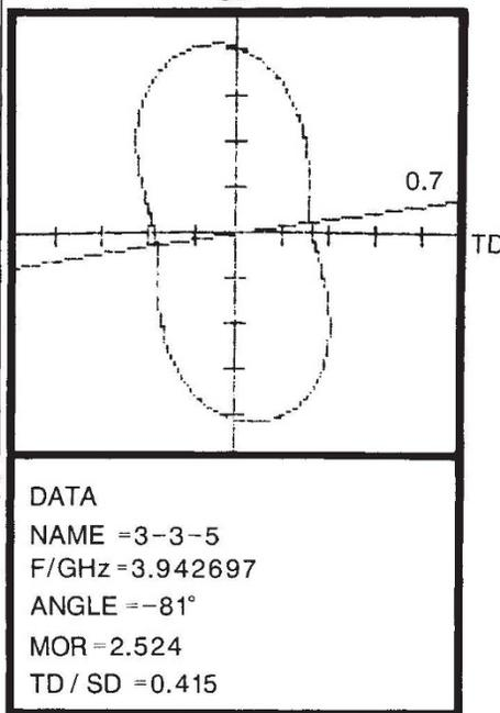
Angular dependence of transmitted microwave intensity at 3.9 gigahertz for a cow leather with a sample size of 100 (length) × 100 (width) × 1.17 mm (thickness) and a weight of 860 gm<sup>-2</sup>. SD, standard direction; TD, transverse direction; MOR, ratio of maximum to minimum intensity (anisotropy).
