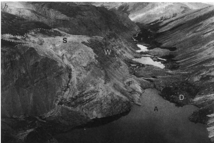
a , Profile of the path of the Avalanche Lake rock avalanche based on 1:50,000 topographic map 95L/6. The pre-landslide topography of Avalanche Lake valley was estimated by projecting the thalweg of the unnamed river that occupies the valley beneath the debris. b , Oblique aerial view (to the west) downstream of Avalanche Lake (A), showing debris in the valley (D), the shelf (S), the wall (W) and a fallback ridge (F) at the wall's base. Debris can be seen on the shelf and secondary run-up, the upper limit of which is delineated by the dashed line, at the shelf's southern margin.
