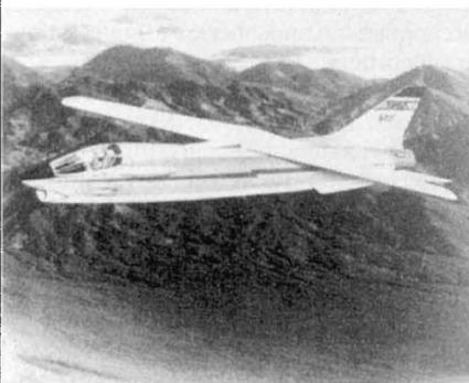
THIS is not a mistake, but what the US aviation company Rockwell intends to do to an F-8 Crusader aircraft. An oblique-wing aircraft, according to aerodynamics theory, might not create a sonic boom at low supersonic speeds. Drag is reduced too, as the lift of the wing is distributed over the long streamwise length. Finally, a boon in naval applications, an oblique-wing aircraft would be much more convenient for stowage in below-deck hangars.
