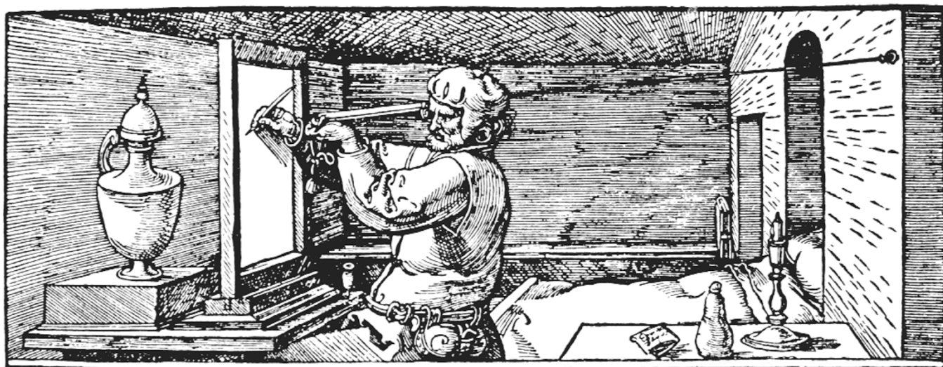
The Artist Takes Aim on a Target for Optical Imitation: one of Albrecht Dürer's "perspective machines", published in his Introduction to Measurement in 1538.
