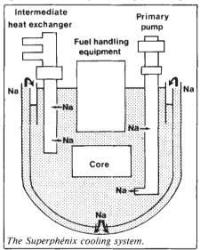
of the cooling circuit, a thin film of sodium passes upwards from the bottom of the main vessel around the outside of the inner jacket, before spilling inwards over the lip of the inner jacket into the core of the reactor. In the first live tests of the cooling system full of heated sodium, the jacket was vibrating with an amplitude of some 12 mm in a diameter of 20 m.
