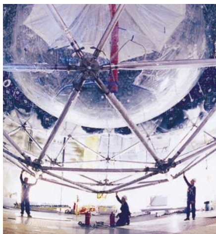
Sun spotter: heavy-water detector could provide clues to the mass density of the Universe.
