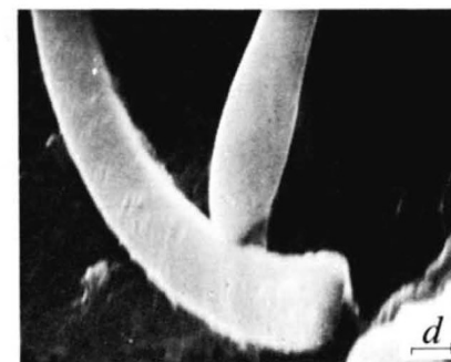
Fig. 1a, SEM of the outside region of manganese-coated coral (V22-D6), showing circular, tubular structures (scale bar, 80 \mu\text{m} ); b and c, SEM of circular structures showing their adherence (b) and cementation (c) to the surface and their tubular nature (scale bar, 8 \mu\text{m} ); d, SEM of tubular structures 2–3 \mu\text{m} in size (scale bar, 1.6 \mu\text{m} ).
