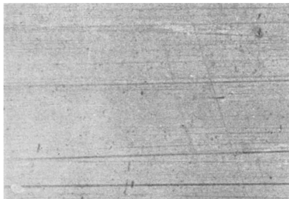
Fig. 3. Sample prepared by means of molecular plating. Polished stainless steel cathode material, solution agitated. ( \times 750 ). No grain visible
