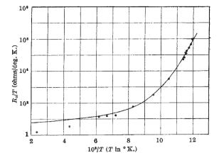
the semiconductor need not imply that the individual barrier heights exceed this value ( $\bar{\varphi}$  for germanium, 1.13 eV.; width of energy gap, 0.72 eV.). Detailed calculations of this sort were not considered worth while, as the data so far available do not justify the inclusion of yet another parameter.
