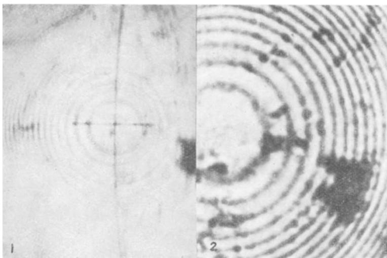
hence Newton's rings can be seen only faintly, superposed on the profile. The radius of curvature calculated from the interference fringes is 0.596 mm. and from the profile 0.595 mm., the estimated error in the latter being some  $\pm 1$  per cent (that is,  $\pm 0.005$  mm.).
