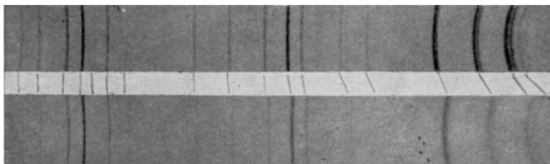
Debye-Scherrer patterns of (above) \eta -carbide ( \text{Fe}_4\text{W}_2\text{C} ) from high-speed steel and (below) extract from an iron-free nickel-base alloy. Manganese K\alpha radiation, 9-cm. diameter camera.
