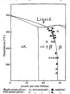
I have now been able to fix this boundary from microscopical examination of alloys annealed and quenched from various temperatures, interpolation from a smooth curve giving the solid solubility limits as follows:
