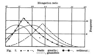
partly of sedimentary, partly of igneous material. contain both types of zircons. Hence elongation frequency curves show two maxima, which may merge to one maximum at an elongation ratio of about 2.0. Other migmatites, having been formed metasomatically, show zircon elongation - frequency curves with only one maximum, at an elongation ratio less than 2.0. Recrystallization of zircon is nowhere evident.
