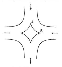
The example, of which details will be given elsewhere, is simply that of two equal and opposite streams approaching one another; each bifurcates symmetrically on meeting, and they depart at right angles to their original direction after pairing off their two halves. At the junction is included a fourcusped wake which may be of any size, or, in the limit, may reduce to a stagnation point. Writing
