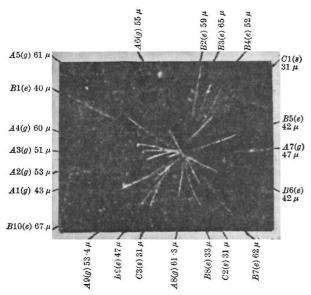
number of grains per division, it seems probable that all the tracks are due to protons. Examination of the tracks under a microscope revealed that the star originated in the mica, and the fact that some of the tracks are somewhat apart from the rest is explained by this, since most travelled directly to the plate, while these few entered laterally.
