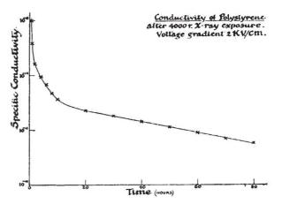
found that the conductivity so induced lingers for a very considerable time after the X-rays have been cut off. The accompanying curve shows the effect during a period of 80 hours following a brief exposure. At the end of this time the material is still far from back to its original state.
