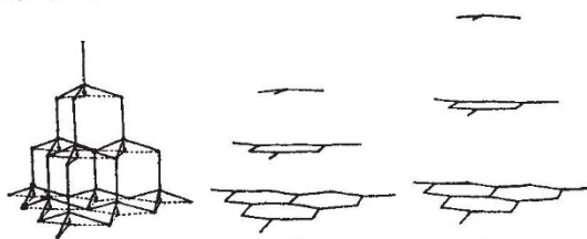
a. Diamond \rightarrow \alpha -pseudo-graphite structure. b. \alpha -pseudo-graphite structure. c. \beta -pseudo-graphite structure.
