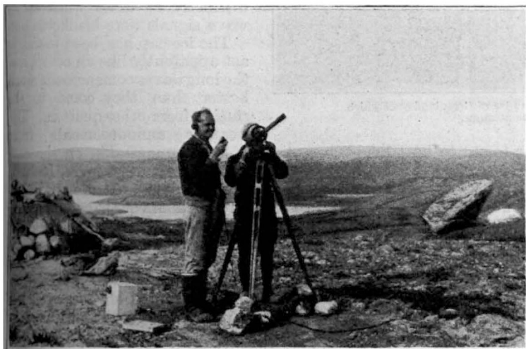
FIG. 2.—Mr. Kallquist, the aerologist, following a balloon with the theodolite at the meteorological station on Mount Evans; Mr. Oscanyan is behind the instrument.
