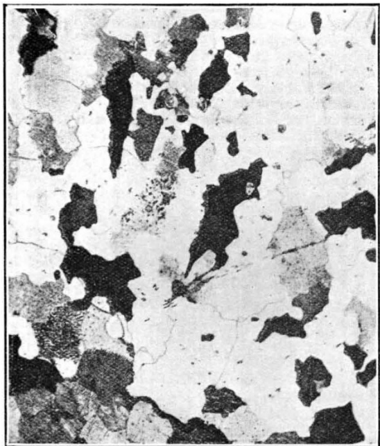
FIG. 1.—Microstructure of pure mercury. Magnification : \times 100 .
