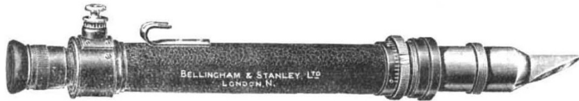
FIG. 3.—Dipping Refractometer (Bellingham and Stanley, Ltd.).
