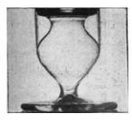
If the original layer of water be too deep, the column will break at its narrowest part, and the same occurs if water be poured gradually into the tube after the column has formed. By varying the width of the vessel, a great variety of shapes may be obtained, all of which are perfectly stable. The water is in all cases displaced from the lower part of the vessel, and bounds the sides of the
