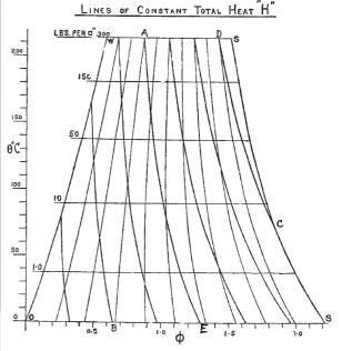
the place of throttling is well protected from loss of heat by a non-conducting covering, and in this case total heat remains constant. Now if the line DC is looked at, it will be seen that steam which is 90 per cent. dry at 300 lb. pressure, if throttled to 150 lb. pressure is about 93 per cent. dry, and if throttled to 50 lb. pressure is about  $95\frac{1}{2}$  per cent. dry. Thus the drying effect is not very great.
