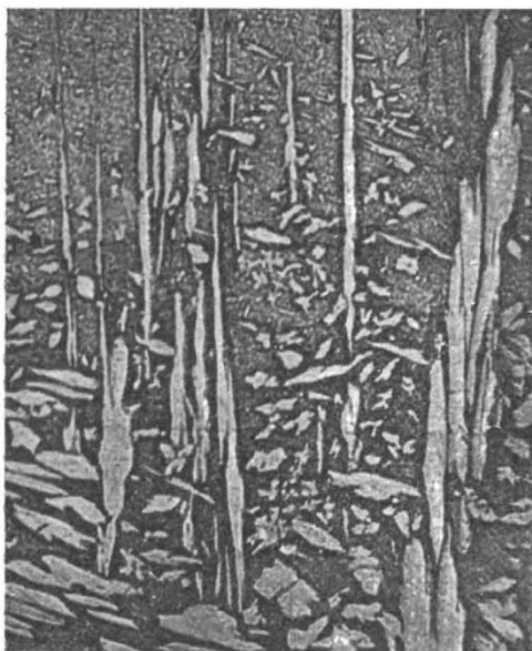
FIG. 3.—Crystals of AlCu_3 .
