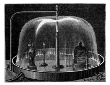
water-height above the jet will be about 60 cm. The flow of the water or its stoppage will of course be regulated by a cock.
