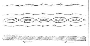
if we imagine the translational velocities at y = 0 and y = a to be in opposite directions, and of such magnitude that the wave velocity is zero; so that we have the case of standing waves. For this case the stream-lines are as represented in the annexed diagram, in which the region of translational velocity greater than wave-propagational velocity is separated from the region of translational velocity less than wave propagational velocity by a cat's-eye border pattern of elliptic whirls.
