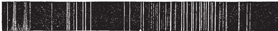
FIG. 4.—Part of the blue region in the spectrum of a mixture of incandescent aluminium, calcium, and iron vapours, showing how the images of the slit produce the appearance of bright lines.
