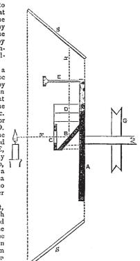
spectrum also moves round the conical screen S S, and when a certain velocity is arrived at, the colours combine and form the original coloured light which is entering at the slit C. In the same way, by using the slides, any two or more colours may be combined to form the resultant colour.
