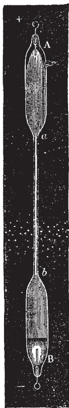
FIG. 24.—Geissler's tube, showing electric discharge.
